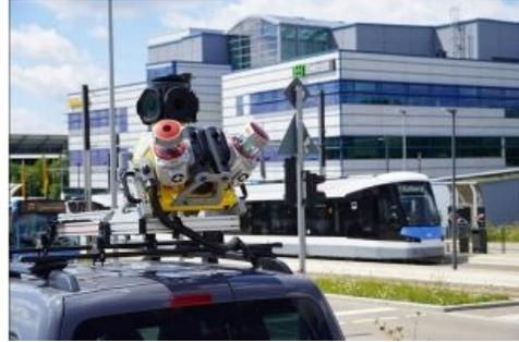
Trimble has recently unveiled the Trimble MX90 mobile mapping system. Integrating advanced Trimble GNSS and inertial technology with Trimble field and office software, the MX90 offers a comprehensive field-to-finish mobile mapping solution. The solution is presented as a new standard in mobile mapping technology, empowering robust workflows for data capture, processing
