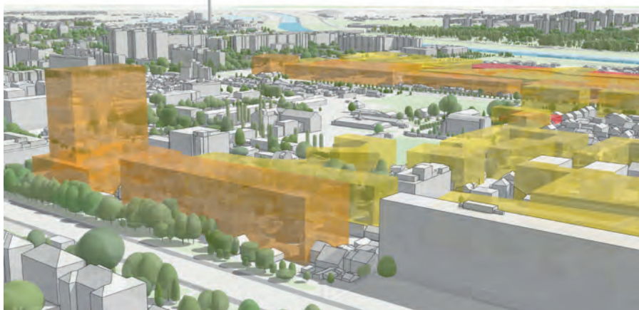
▲ Figure 3: 3D building outlines and volumes interpreted from a detailed urban plan (Trnje, Zagreb).
