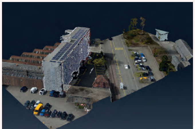
▲ Colourized point cloud.
