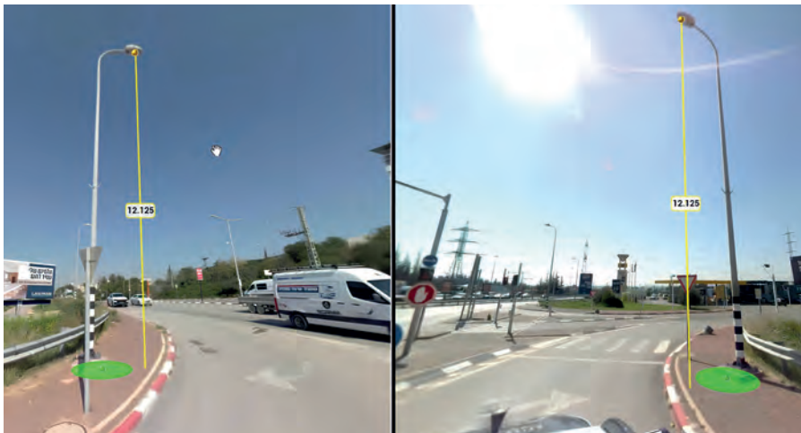
▲ The measured height of lighting pole using the mobile mapping system.
