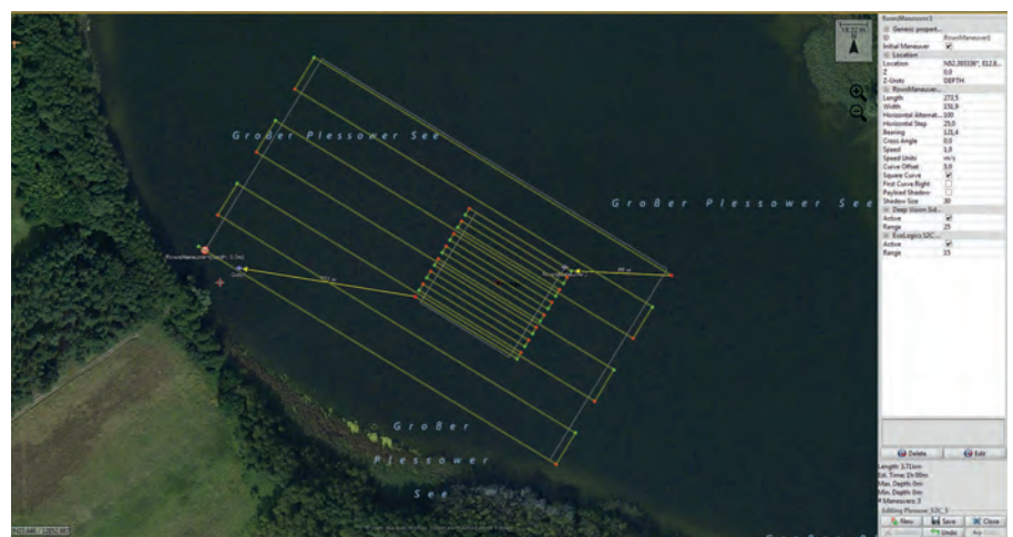
▲ Figure 1: Example of a survey plan EvoLogics performed at Plessower Lake in 2017.
