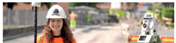
▲ Innovations such as the Leica AP20 AutoPole can help surveyors stay ahead of the curve by increasing productivity and allowing them to measure points that were impractical or unsafe to measure before.
