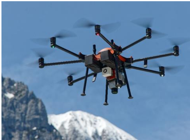
Soleon LasCO 1 with RIEGL miniVUX-3 UAV
