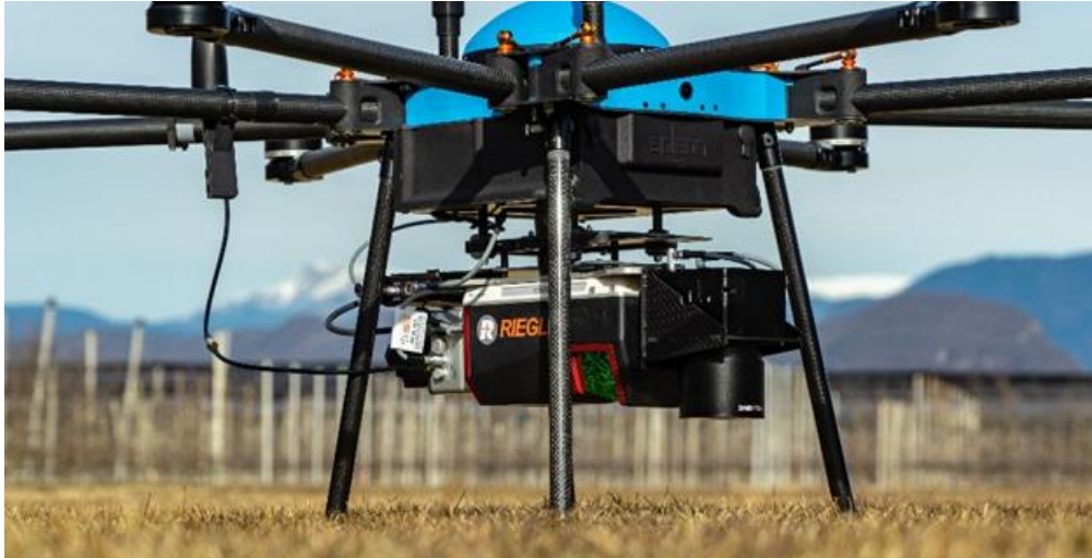
Soleon LasCO 2 with RIEGL VUX-120 and PhaseOne iXM100
